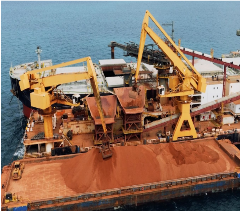
Figure 8: MMI's bauxite on a barge being loaded to a capesize vessel by the Ikamba offshore floating terminal
