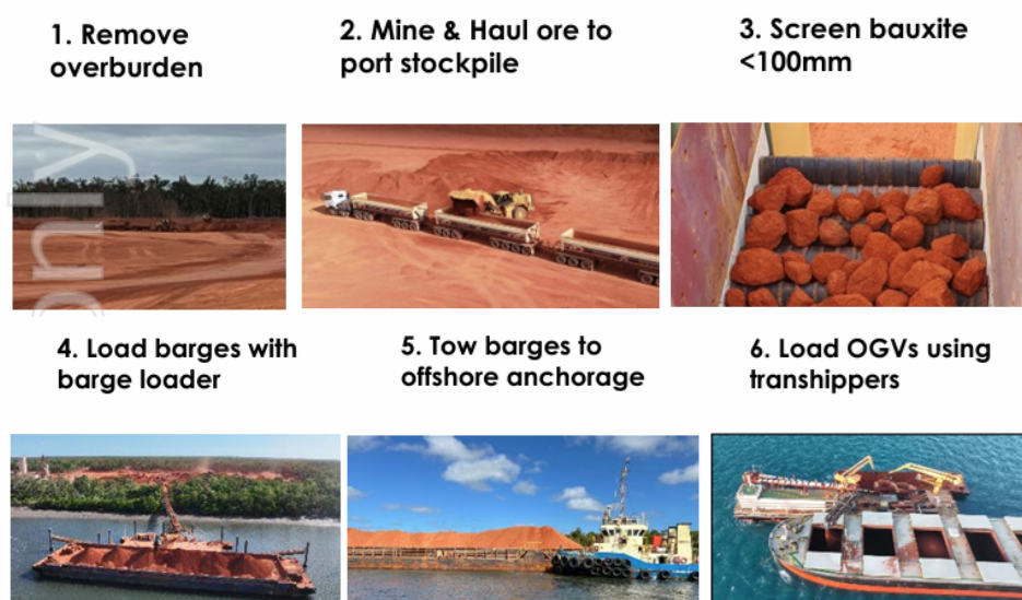
Figure 1: Schematic of pit-to-ship logistics chain
