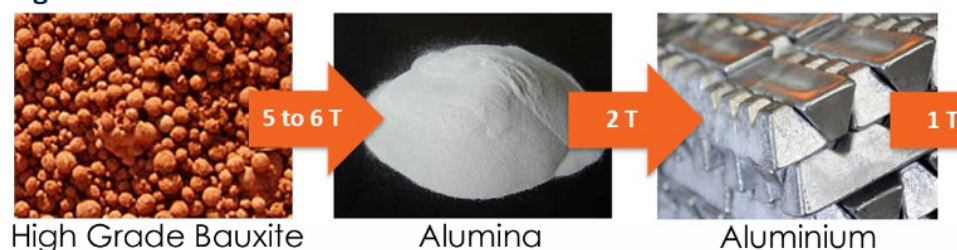
Figure 4: bauxite is feedstock for aluminium metal via alumina
