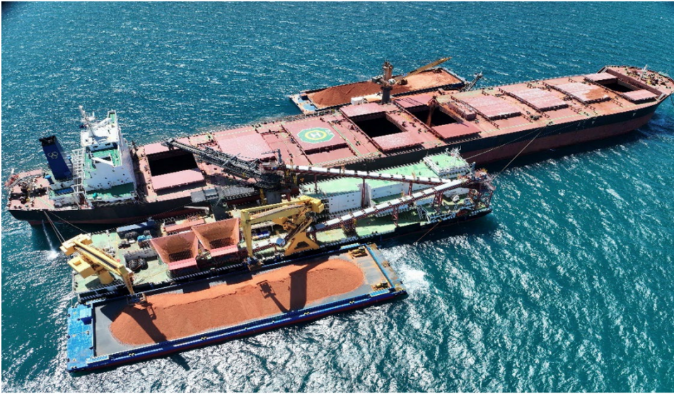
Figure 38: Cape vessel loading with Ikamba (near side) & floating crane.
