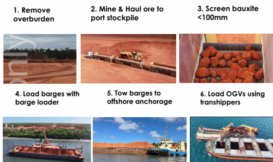
Figure 5: MMI's schematic of pit to ship logistics chain
