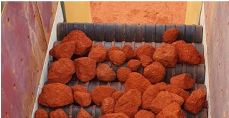
Figure 39: Screened bauxite with wobbler blocking cemented oversize
