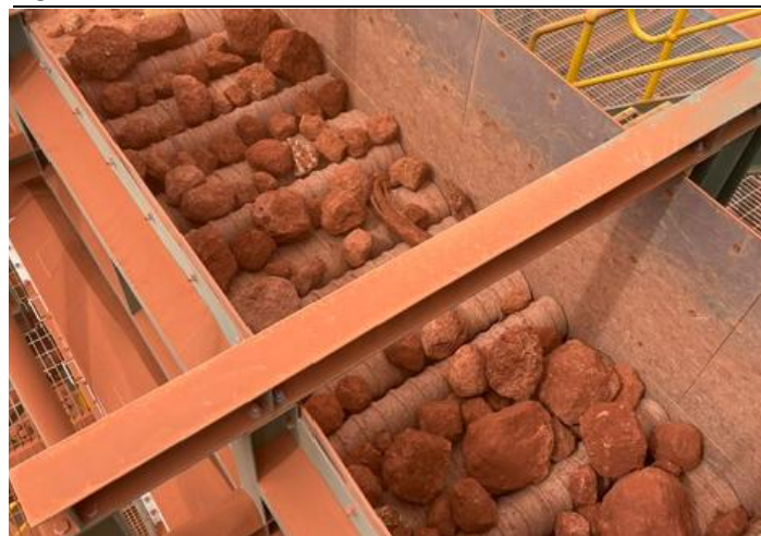
Figure 2: Wobbler screen to remove oversize material
