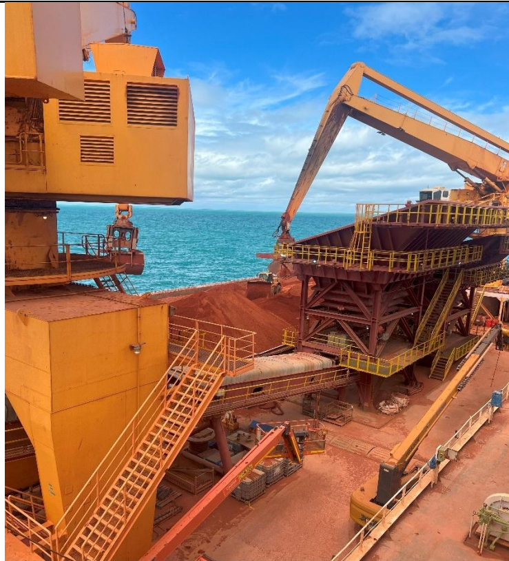
Figure 7: OFT showing two cranes loading bauxite from barge into chutes for transfer via conveyor onto the Newcastlemax ship
