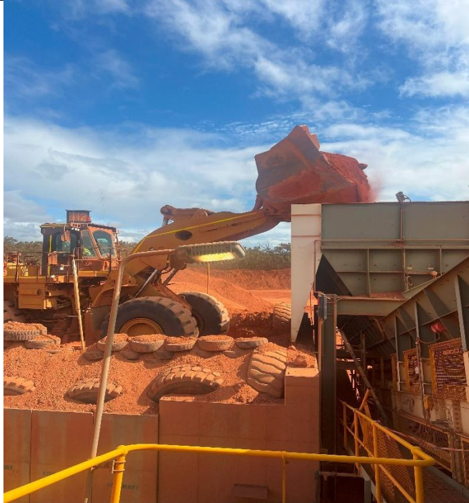
Figure 3: Bauxite being loaded for screening and conveyer to barges
