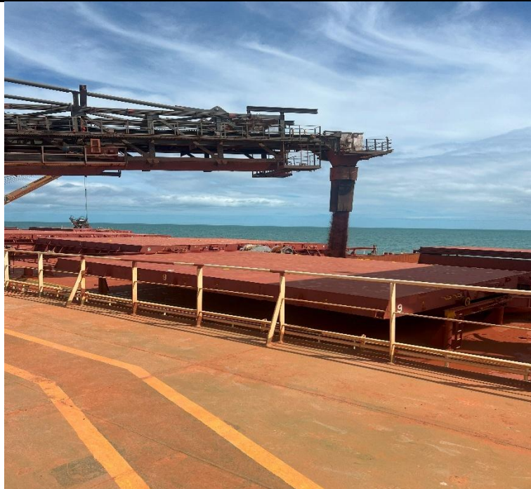
Figure 8: OFT ship loading boom transferring bauxite into Newcastlemax cargo hold
