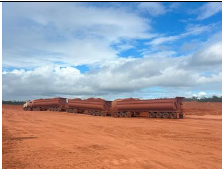
Figure 2: Scania truck with triple trailer (180t) being loaded with bauxite
