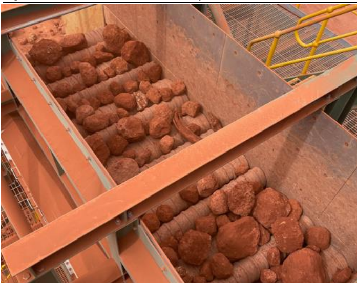
Figure 3: The new wobbler screen in operation
