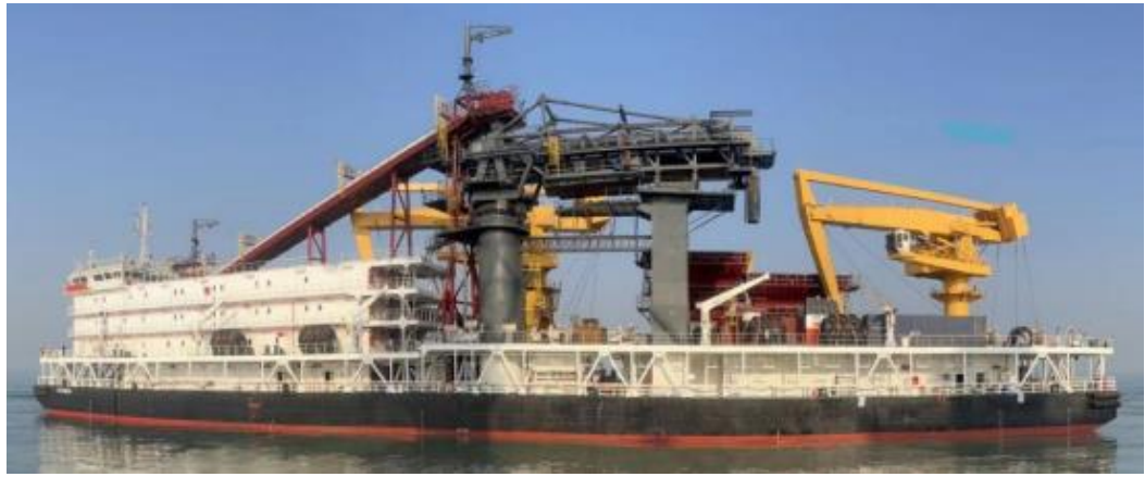
Figure 3: Ikamba OFT – rated capacity of 9Mtpa
